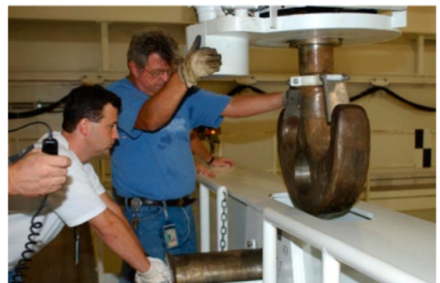
Technicians prepare to install a huge locking pin through the spreader bar and crane hook used to rotate the payload canister in the CRF.
