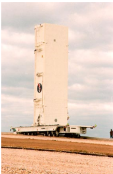
The STS-110 payload -- S0 truss for the International Space Station -- is transported to the pad inside the payload canister.
